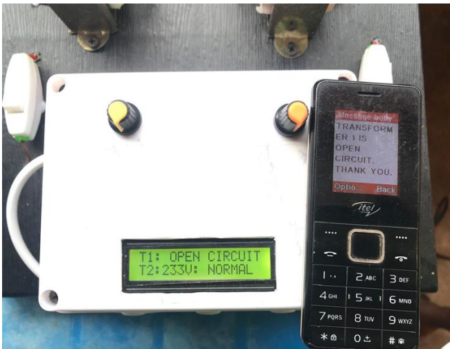
Fig. 14 The picture of the implemented system of transformer 1 in an open circuit state
