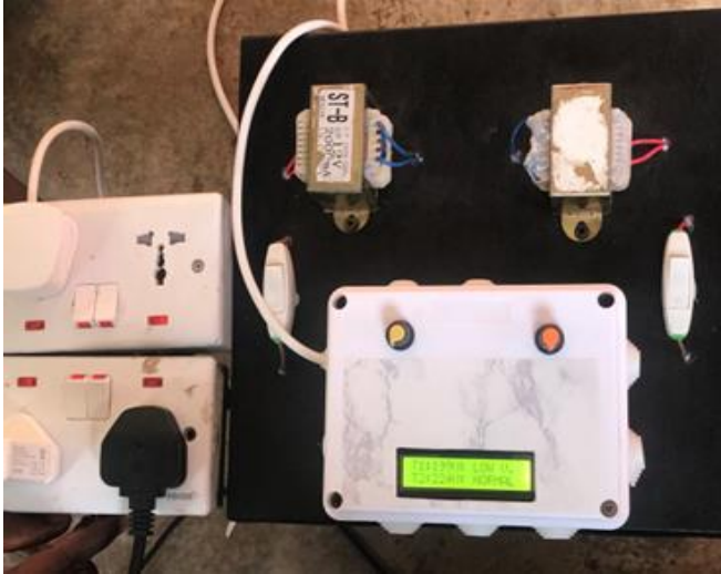
Fig. 4 Final packaging of the distribution transformer monitoring system
