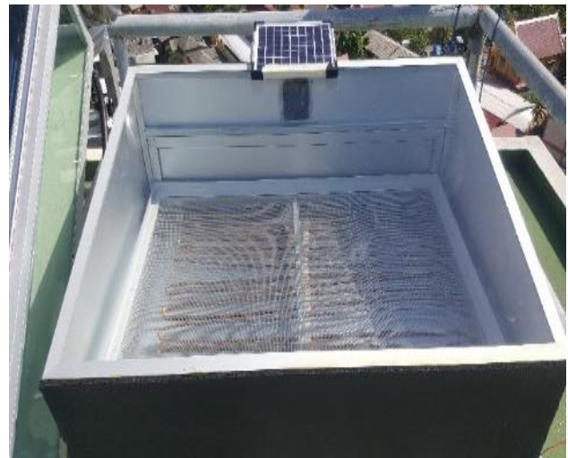
Fig. 4 New solar drying cabinet and pulsing heat pipes' placement
