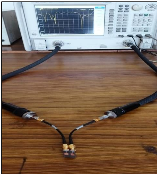
Fig. 21 Measurement of S-parameter of fabricated 2x2 MIMO
