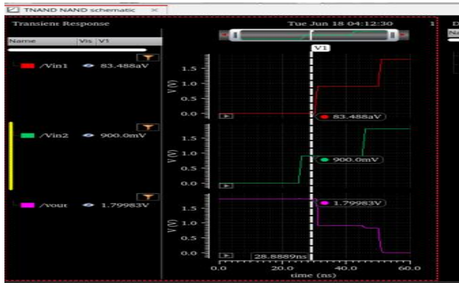
Fig. 17 Transient response of TNAND and TNOR gates
