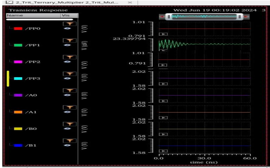
Fig. 22 Output response of 2 trit multiplier
