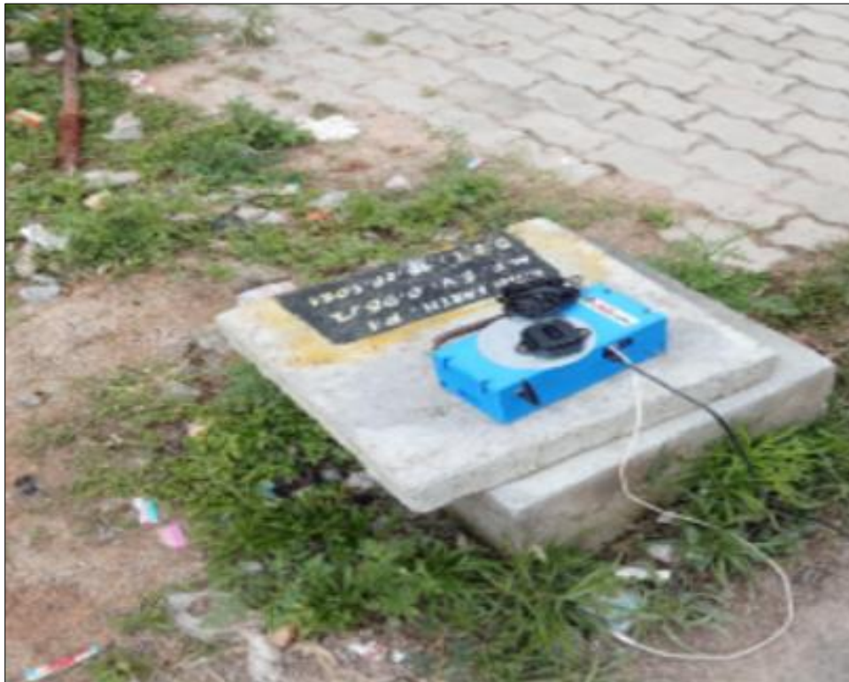
Fig. 4 IoT positioning kit placed at remote farmland
