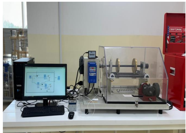
Fig. 2 Integration of MFS with LabVIEW software
