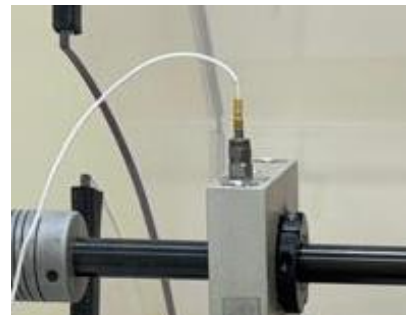
Fig. 5 Vertical mounting of the accelerometer on the rotating shaft
