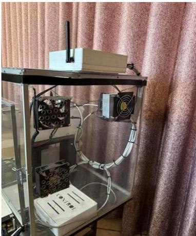
Fig. 32 Temperature and ventilation control system
