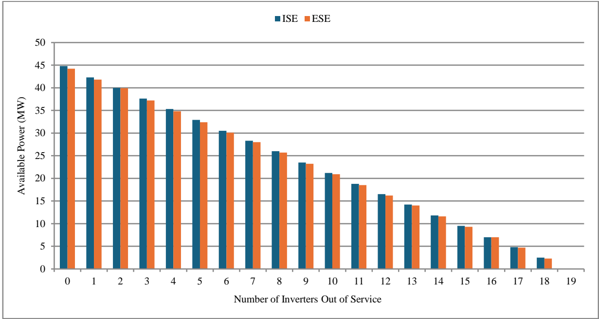
Fig. 8 ISE and ESE vs. Number of Inverters Out of Operation-Monofacial Case
