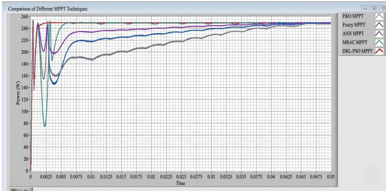
Fig. 12 The PV output power using different MPPT controllers (Scale 0 to 0.05)
