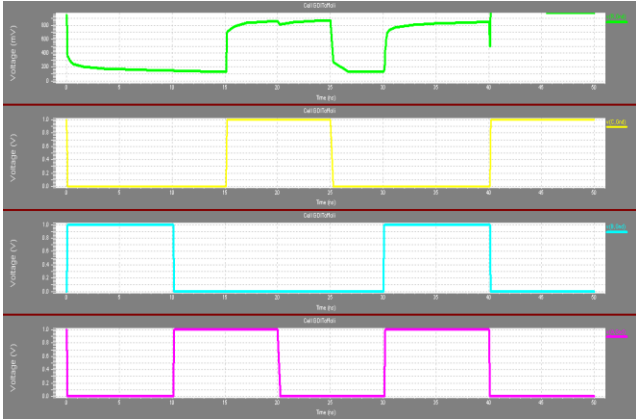
Fig. 8b) Simulation results for Toffoli Gate using GDI.
