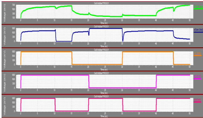
Fig. 15b) Full Adder using proposed RGG and PRGG1 gate
