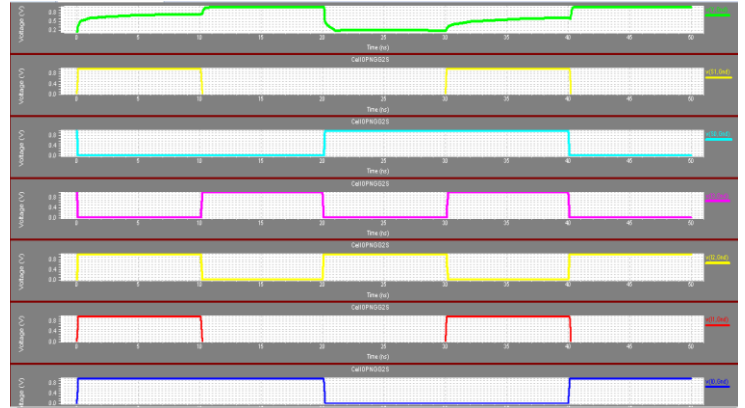
Fig. 17b) Simulation results for 4:1 Multiplexer
