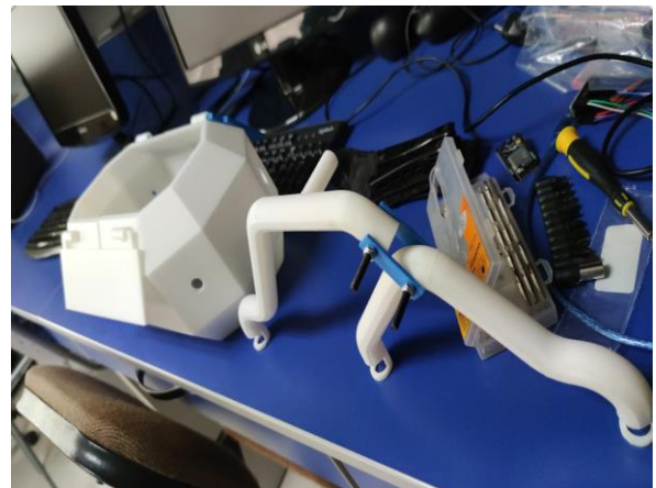
Fig. 6 Fully assembled chassis and rocker-bogie suspension system
