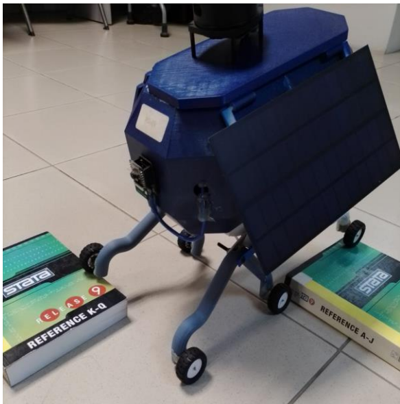
Fig. 14 Rover during mobility tests in autonomous mode
