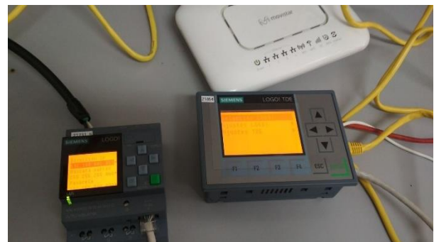
Fig. 7 PLC and HMI configuration
