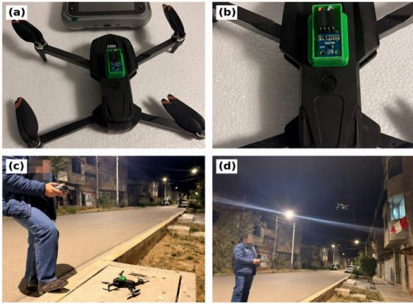
Fig. 2 UAV-IoT platform used for illuminance measurement: (a) UAV with the installed sensor module, (b) Detail of the BH1750 mounting, and (c) and (d) System deployment during the nighttime campaign.
