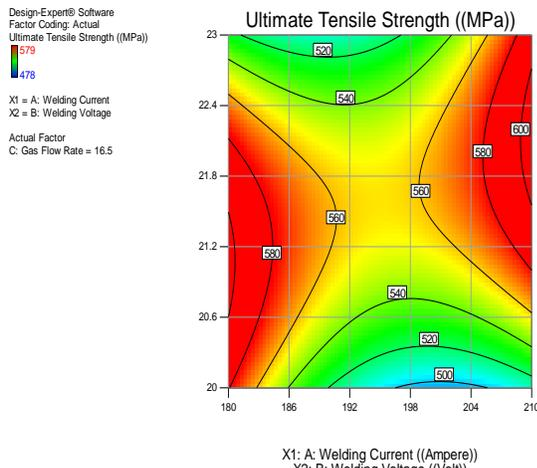
**Fig. 3 Contour Plot of the Ultimate Tensile Strength: Welding Current vs. Voltage**
