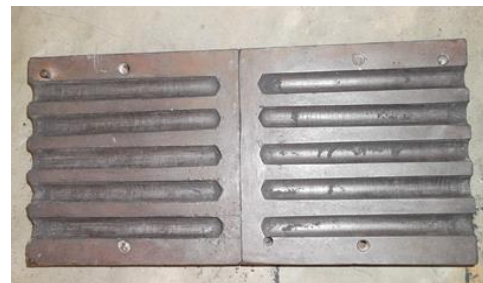
Fig. 4 Grey cast iron mould
