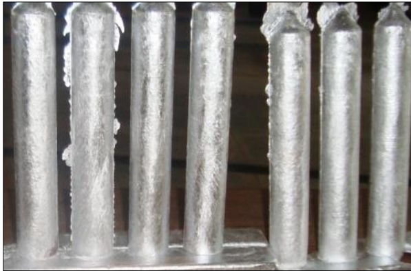
Fig. 6 Cast fingers of the base alloy Al-4Mg
