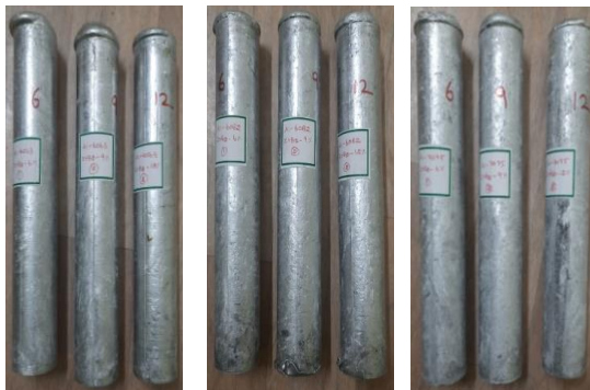
Fig. 3 (b) Stir casted Al MMNC billets (Al-6063, Al-6082, Al-7075) with 6%, 9% and 12% ZrB_2
