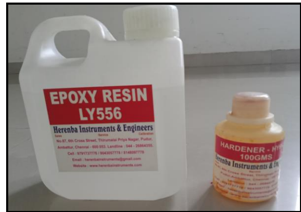
Fig. 1 LY556 epoxy and HY951 hardener
