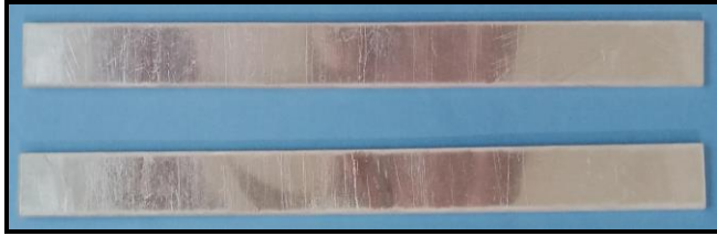
Fig. 4 0° fiber orientation specimens of size 250 mm (L) x 15 mm (B) x 1.8 mm (t) were cut from FMLs sheet
