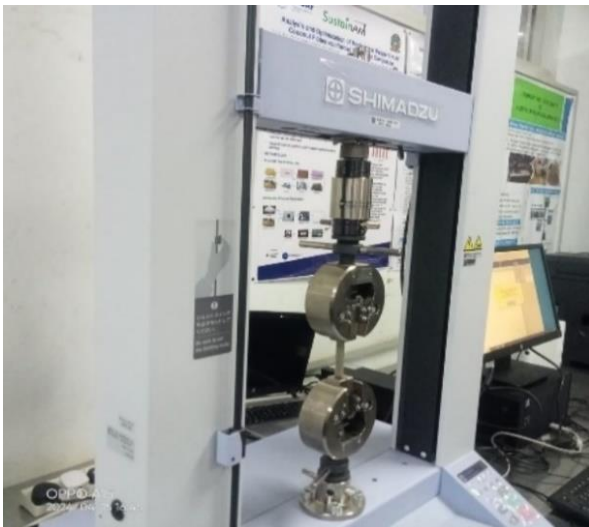
Fig. 5 Tensile sample mounted on universal testing machine
