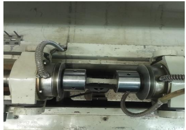
Fig. 6 Fatigue sample mounted on ONO's High-Temperature Bending Fatigue Testing Machine Model 7
