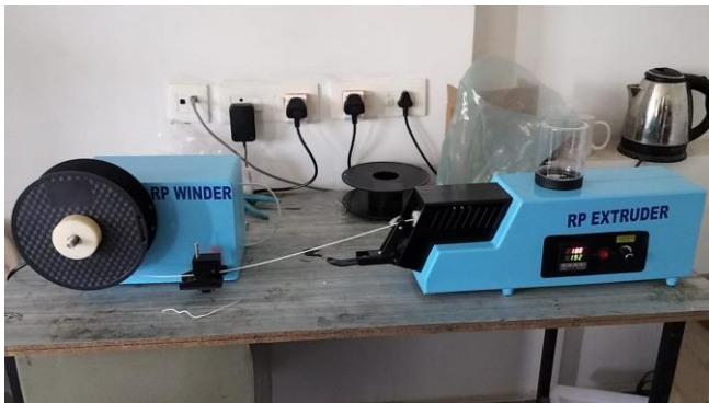
Fig. 2 Composite filament making process
