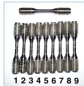
Fig. 3 Un-notched (top) and notched (1-9 below) fatigue specimens
