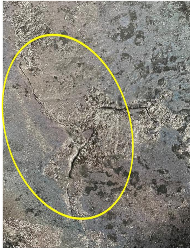
Fig. 6 Defect found in casting component
