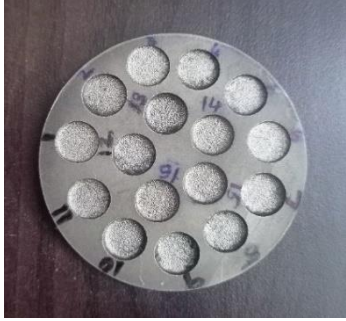
Fig. 2(c) Workpiece operated with used vegetable oil as dielectric fluid
