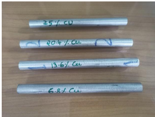
Fig. 1 Al2021 Electrodes with varying % of Cu
