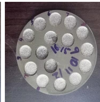
Fig. 2(b) Workpiece operated with used gear oil as dielectric fluid
