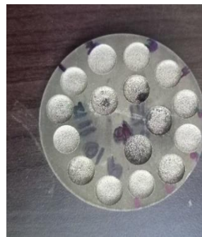
Fig. 2(a) Workpiece operated with EDM oil as dielectric fluid
