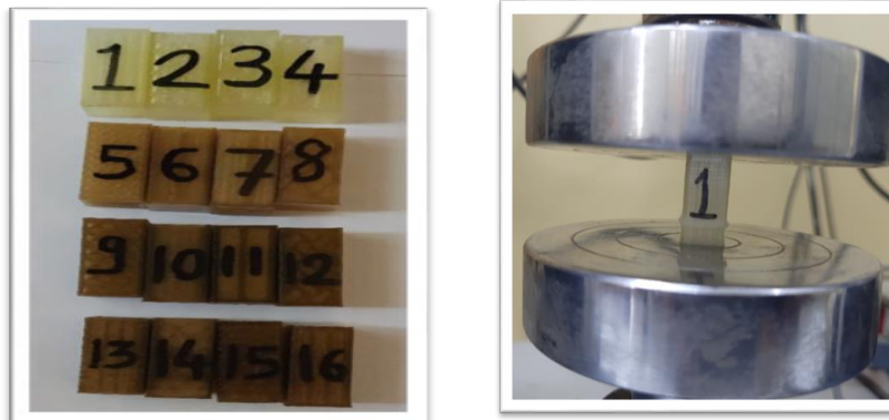
Fig. 8 3D printed specimen and compression test
