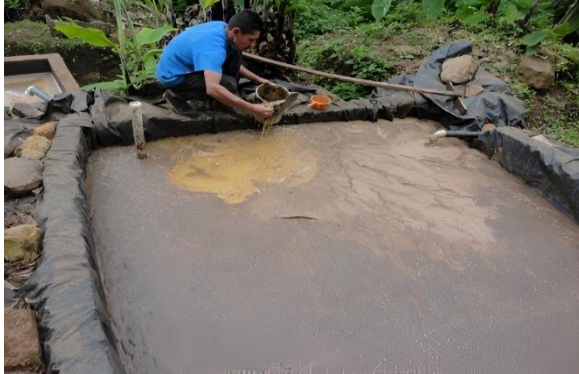
Fig. 1 Manual separation of honey waters through sedimentation in the province of Chanchamayo
