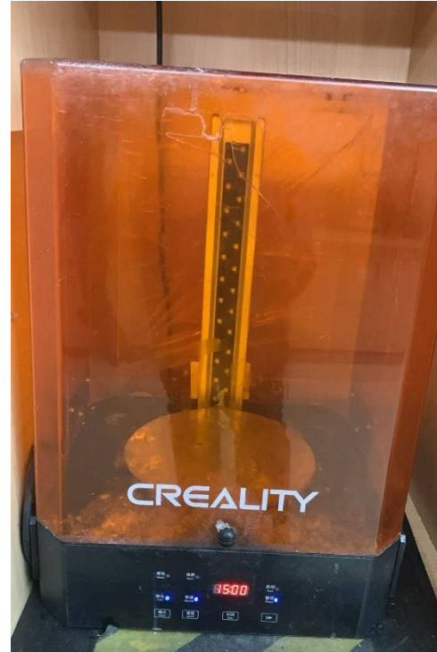
Fig. 23 SLA-based 3D printer and UV curing machine
