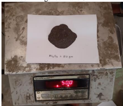
Fig. 4 Weighing of Al 2 O 3 = 50 gms powders for mixtures
