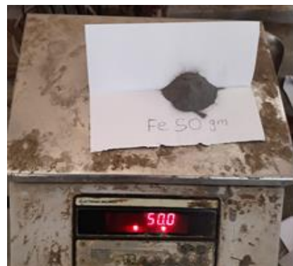
Fig. 5 Weighing of Fe = 50 gms powders for mixtures
