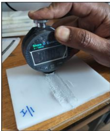
Fig. 3 Shore D hardness testing
