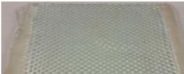
Fig. 2 Glass fibre reinforced laminate material
