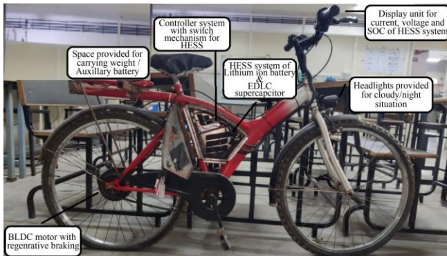
Fig. 10 Final e-bicycle with HESS system
