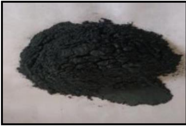
Fig. 3 Tungsten Carbide (WC) powder used as reinforcement
