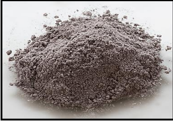
Fig. 2 Al6061 alloy used as matrix material
