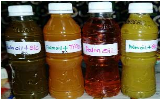
Fig. 1 Prepared samples of hybrid nanofluid
