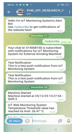
Fig. 14 Threshold exceed limit notification in mobile application
