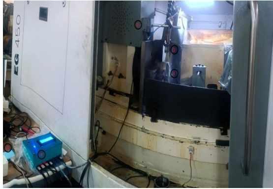
Fig. 8 Experimental Setup, (1) Bearing race (2) IR Thermometer (3) Magnetic stand (4) Control unit with screen (5) Wi-fi router [4, 5, 7]
