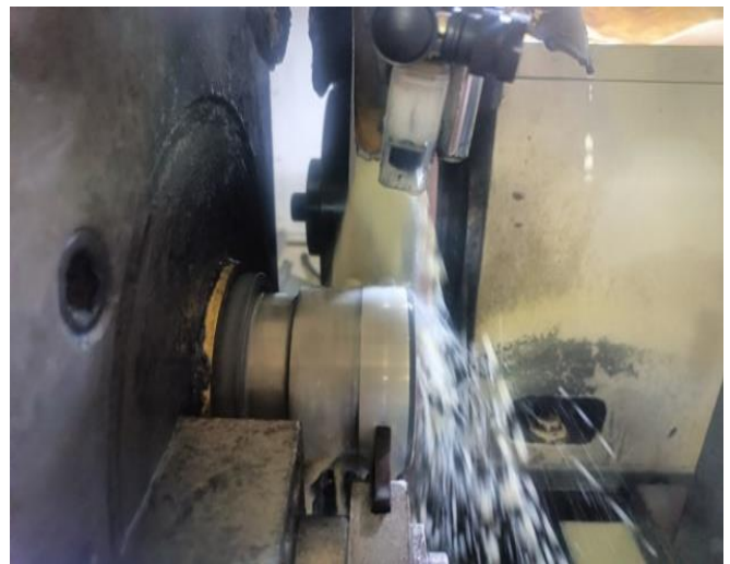
Fig. 7 IR Thermometer sensor attached near the cutting zone
