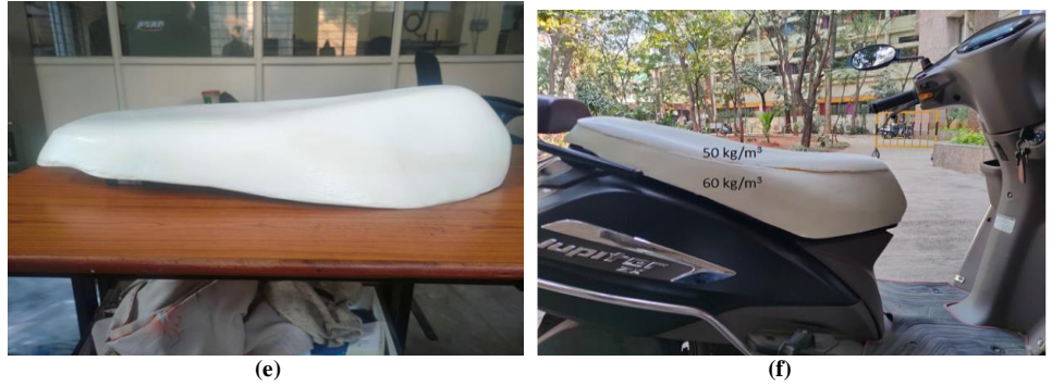
Fig. 3 Different foam configurations (a) Seat with no foam, (b) 30 mm thickness and 60 kg/m 3 density foam seat, (c) 40 mm thickness and 60 kg/m 3 density foam seat, (d) 50 mm thickness foam seat 60 kg/m 3 density foam seat, (e) 40 mm thickness and 50 kg/m 3 density foam seat and (f) Multilayer foam density (50-60 kg/m 3 ) with an overall 40 mm-thick foam seat.
