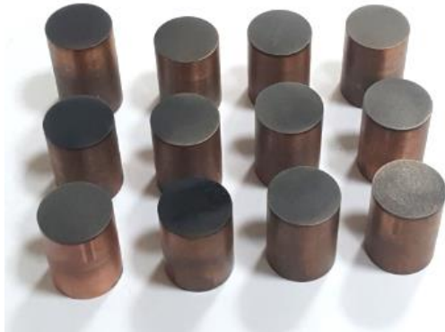
Fig. 7 Copper electrode surface after EDM process
