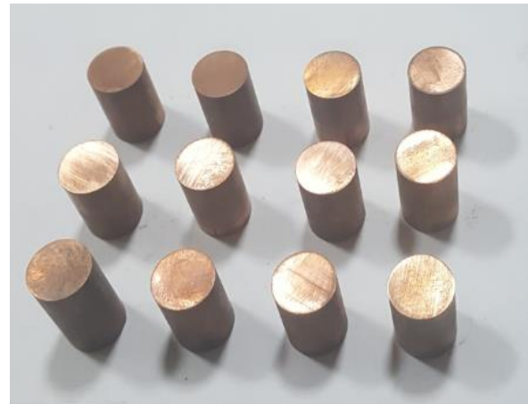
Fig. 3 Copper electrode, \varnothing 15 mm
