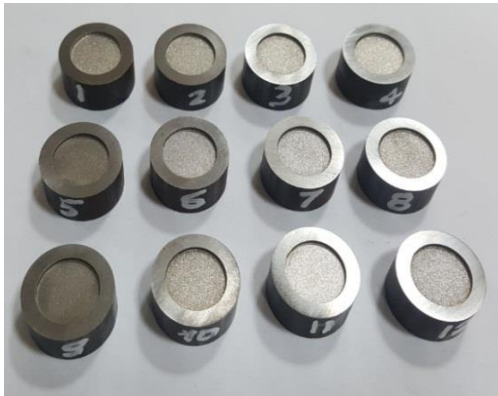
Fig. 6 9XC steel surface after EDM process
