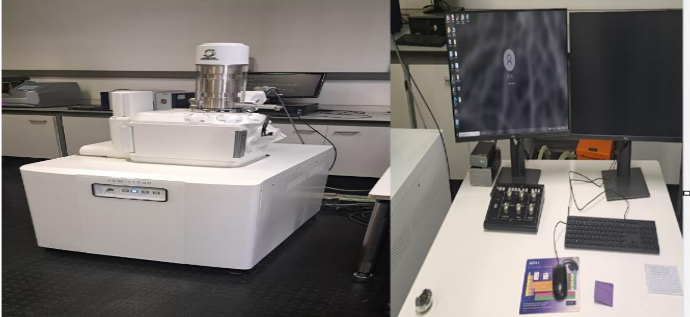
Fig. 7 JSM IT500LA JEOL SEM Scanning Electron Microscope
