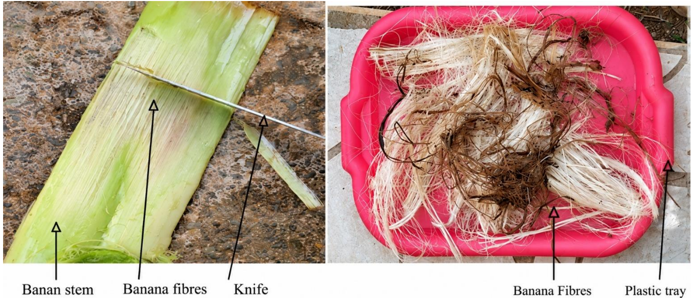
Fig. 2 (a) Extraction process of banana fibers, and (b) Drying banana and hemp fibers.
