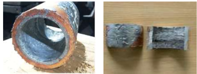
Fig. 5 (a) Bimetal Cylinder casted in Horizontal centrifugal casting machine at 600rpm (b) Bimetal Cylinder Cut in half.
