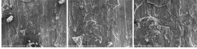
Fig. 15 SEM images of bimetal specimen D (without insulation) at marked position X1 as shown in Fig. 6(d)
