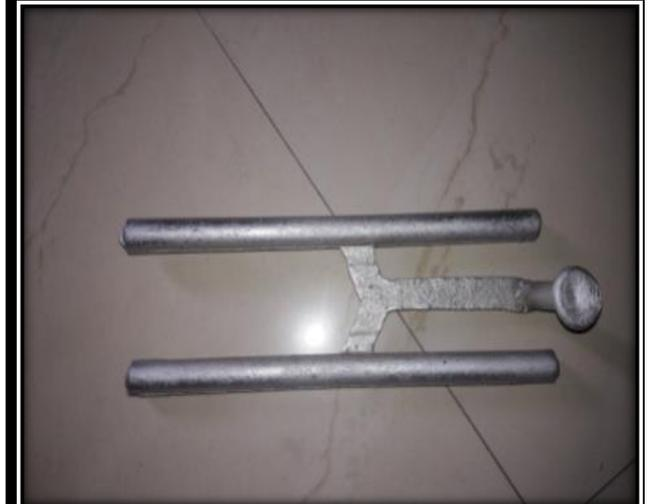
Fig. 9 Formed Aluminium 7075 Hybrid Metal Matrix Composite
