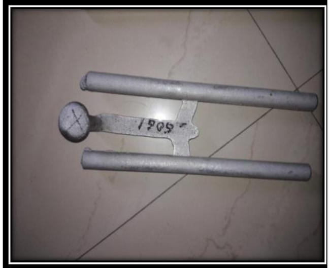
Fig. 8 Formed Aluminium 6061 Hybrid Metal Matrix Composite
