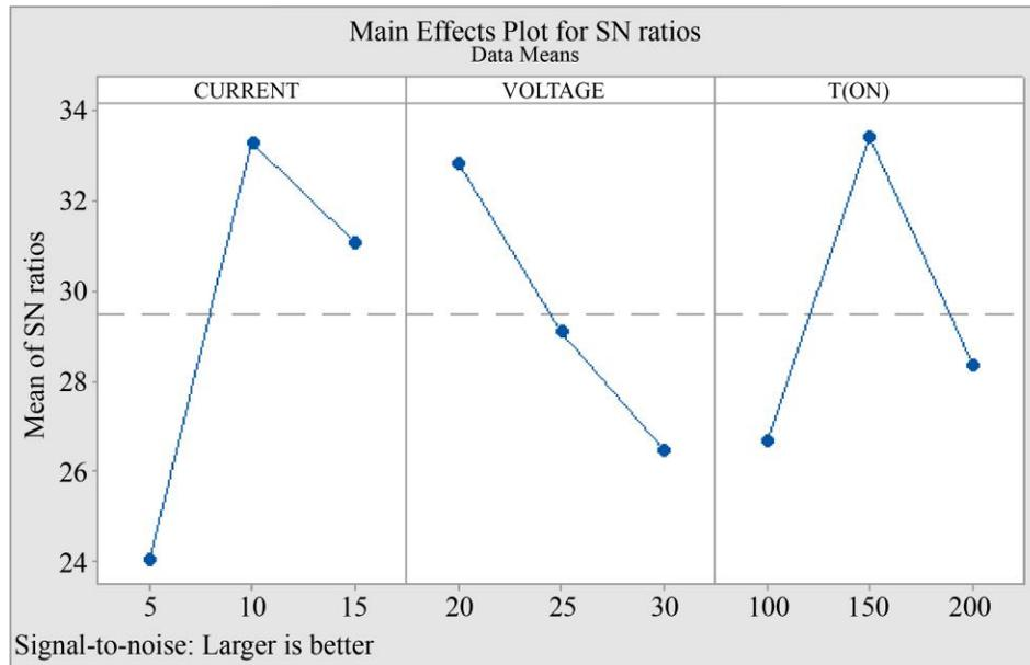
Fig. 16 SN ratio plot for “MRR”
