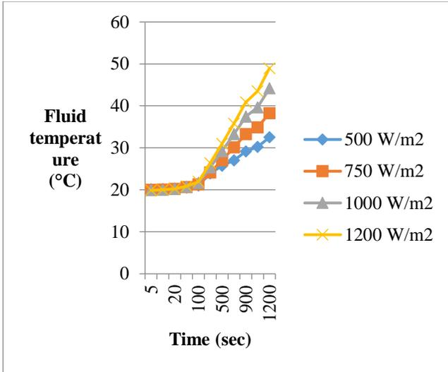
Fig. 9 Fluid temperature exiting the thermal pipes at the PV-Thermal Solar Collector.
