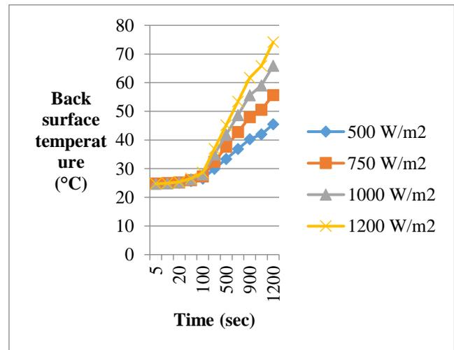
Fig. 8 Back PV Cell temperature at different solar radiation
