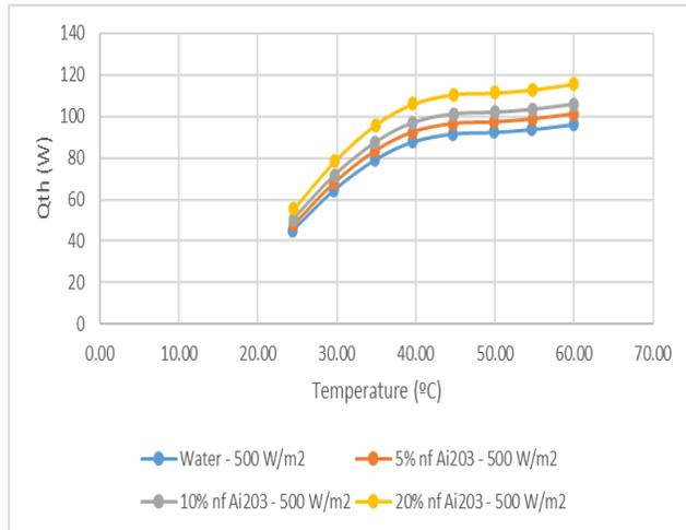
Fig. 2 Thermal Energy PV-Thermal collector at different Heat transport fluid temperatures
