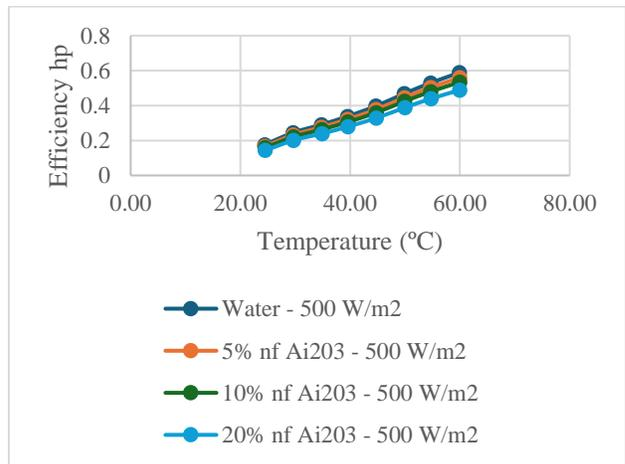
Fig. 4 Heat Pipe thermal efficiency
