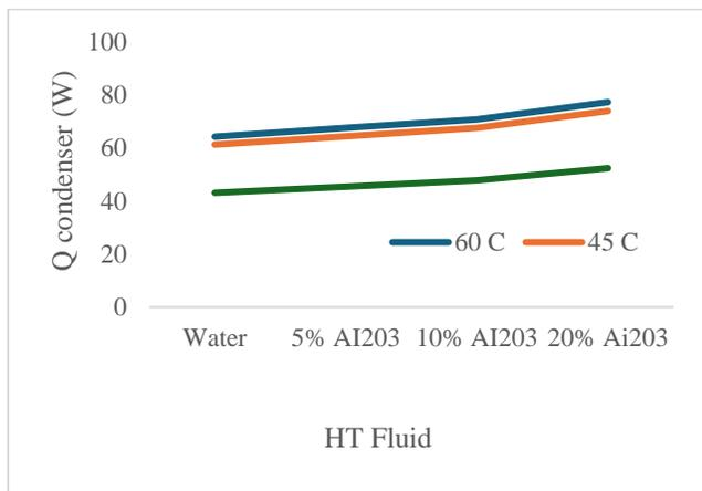
Fig. 7 Heat Pump Condenser thermal energy at different temperatures
