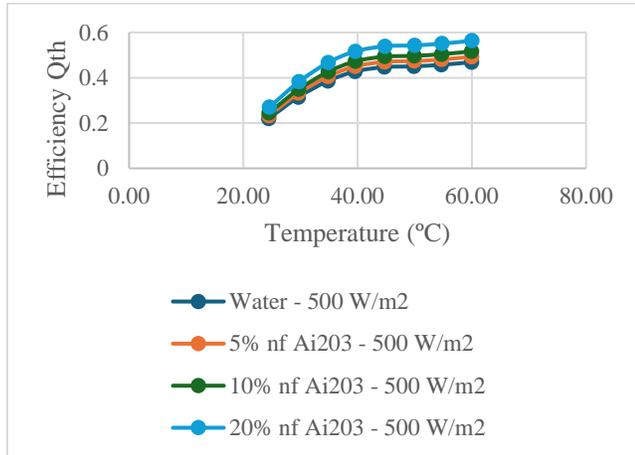
Fig. 5 Integrated thermal efficiency at PV thermal-heat Pipes system
