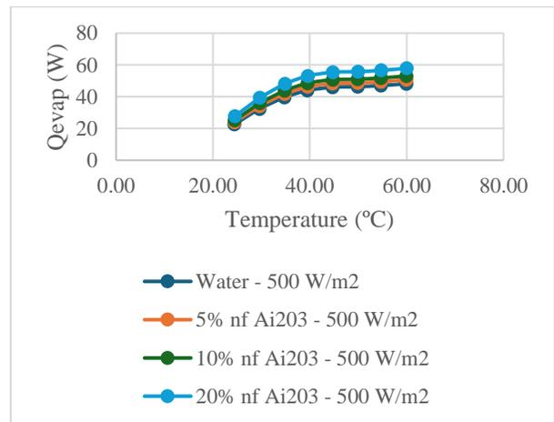
Fig. 3 Heat pipe Evaporator thermal energy
