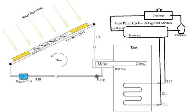
Fig. 1 PV/Thermal-Heat Pipe hybrid system
