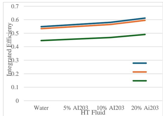
Fig. 11 Integrated efficiencies at Solar 750 irradiances (w/m²)
