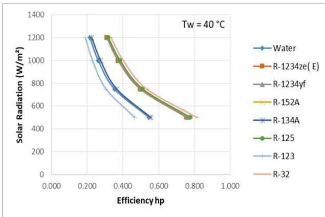
Fig. 10 Hear pipe efficiency at different working fluids.
