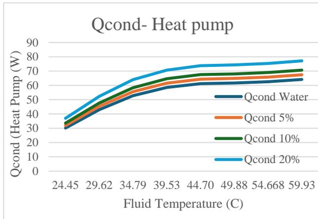
Fig. 6 Heat Pump Condenser thermal energy at different concentrations
