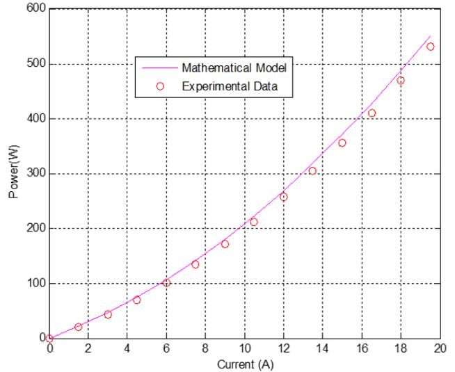
Fig. 13 Comparison between model and experimental data [17, 30]
